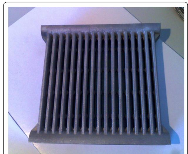
Figure 7 Side view of the heat exchanger.
