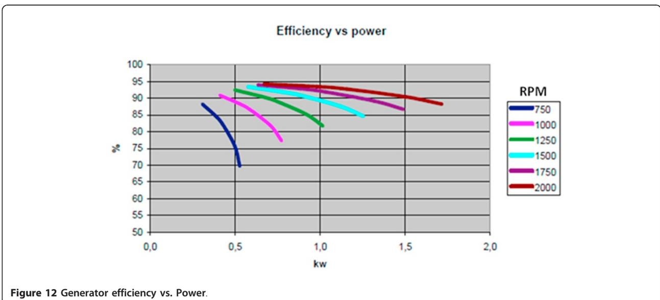
Figure 12 Generator efficiency vs. Power.
