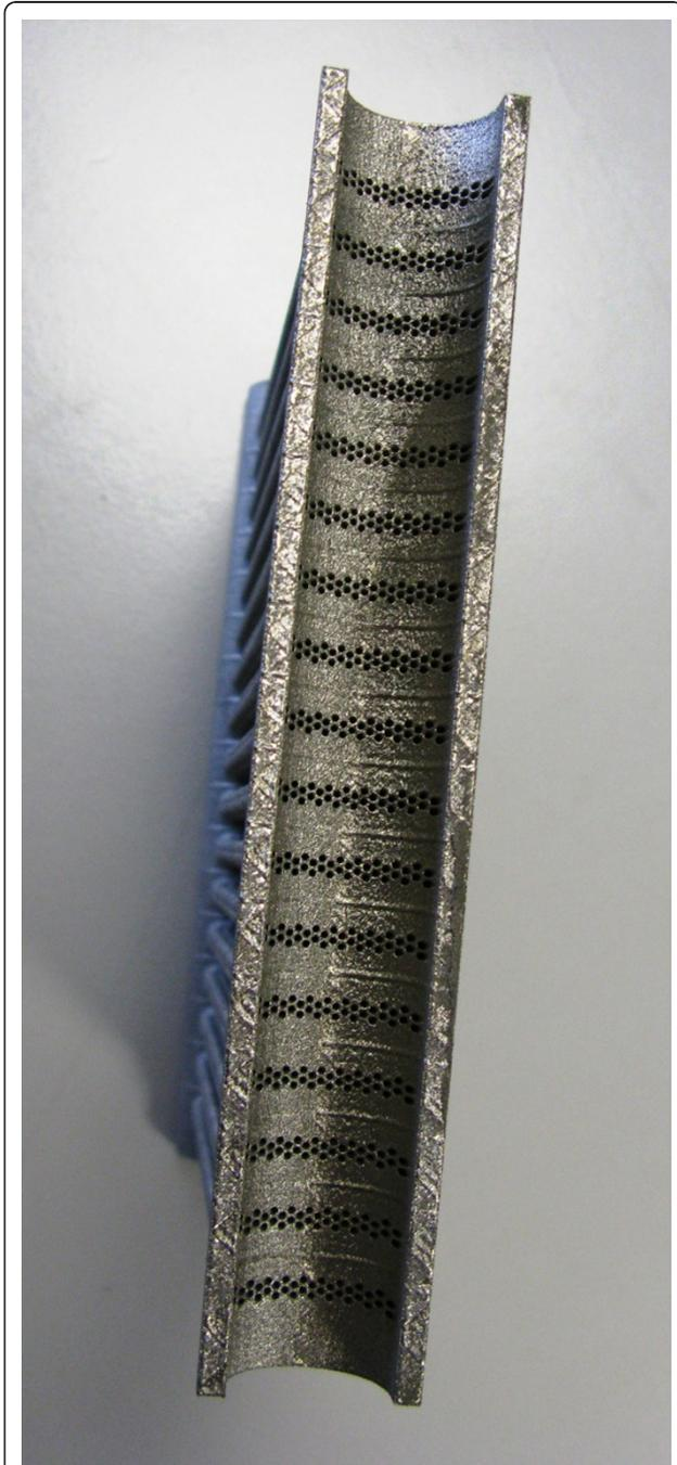
Figure 6 Top view of the heat exchanger from the manifold.
