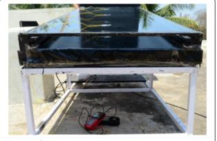
9 am to 5 pm. The solar radiation was measured using pyranometer. The K-type thermocouples were used for
