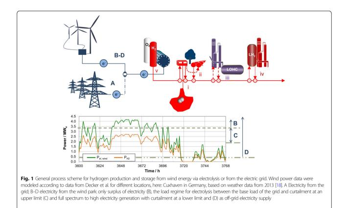
Modes B, C, and D represent the renewable modes and are therefore combined in the general process scheme. The differences between the different modes are explained using the example wind power data presented in the lower part of Fig. 1.
