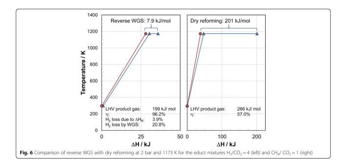
of the reaction. The  $H_2$  balance of rWGS shows that a high share of 20.8% is lost by the chemical reaction and only 3.9% of the hydrogen can be used for the heat supply if this would be taken into account for delivering the heat of reaction of rWGS. Figure 6 visualizes the above-presented comparison between the two process routes.
