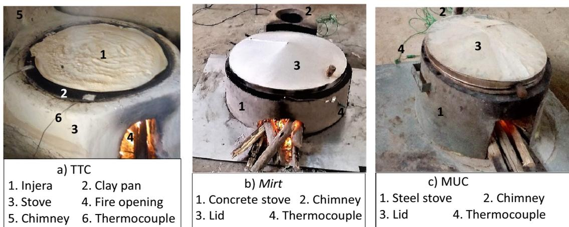
**Fig. 1** Stoves under controlled cooking tests: **a** traditional Tigray stove, **b** Mirt stove and **c** MU prototype stove
