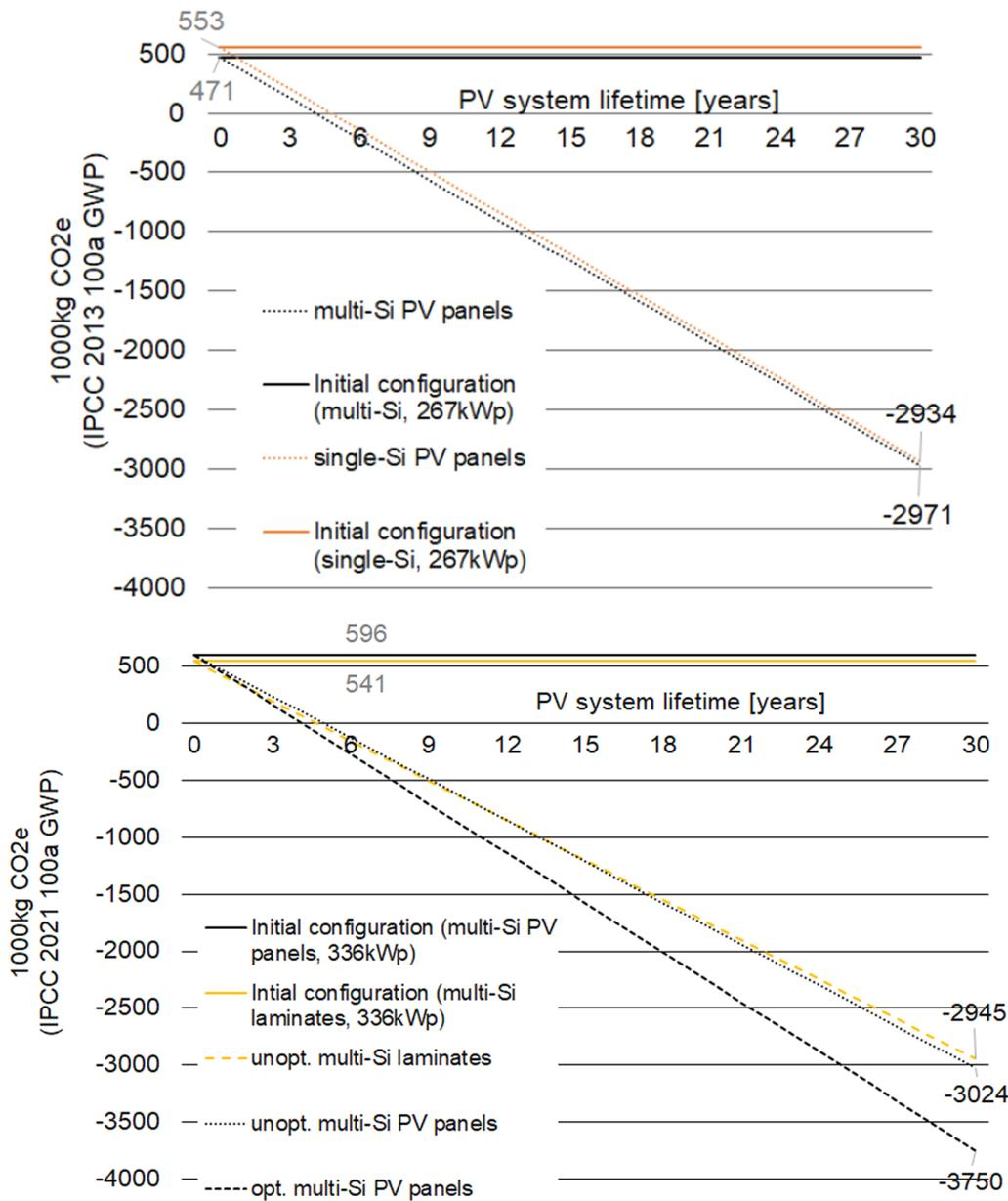
**Fig. 8** CO<sub>2e</sub> break-even-point analysis for case 1 (flat roof, 267 kWp) and case 2 (slanted roof, 336 kWp)
