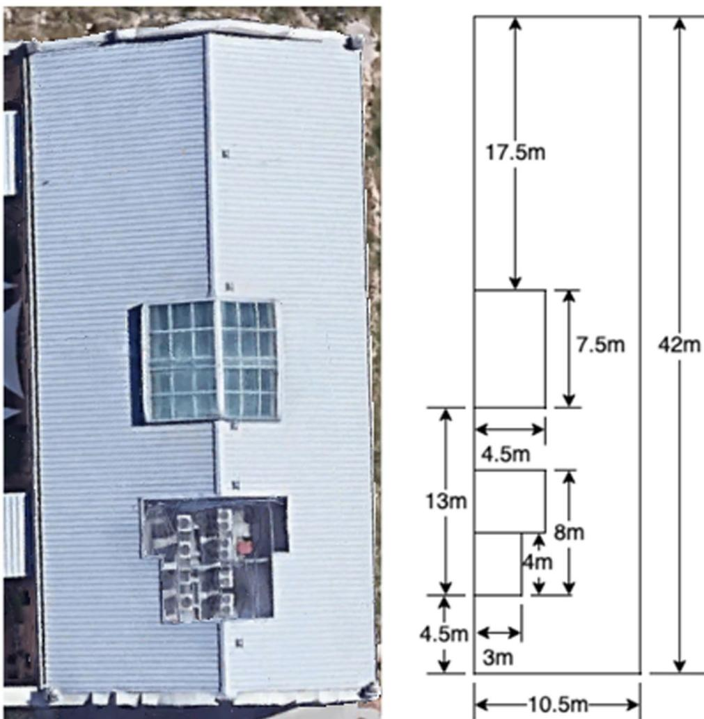
**Fig. 3** Drawing and picture of the rooftop of case 2
