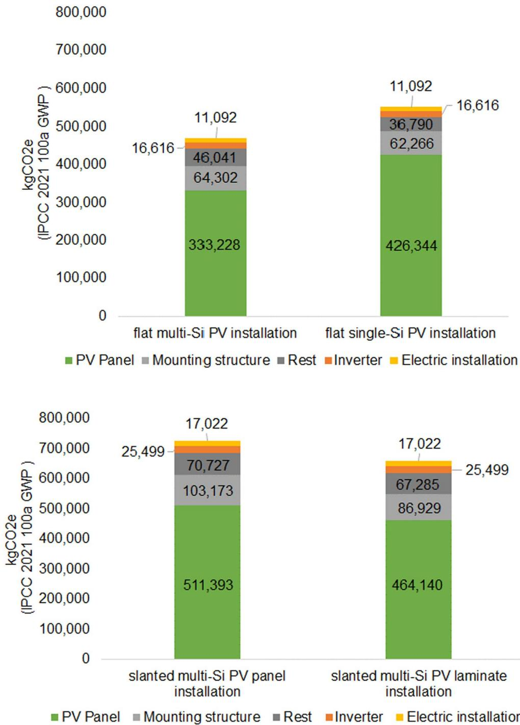
**Fig. 6** GHG emissions of PV components for cases 1 and 2
