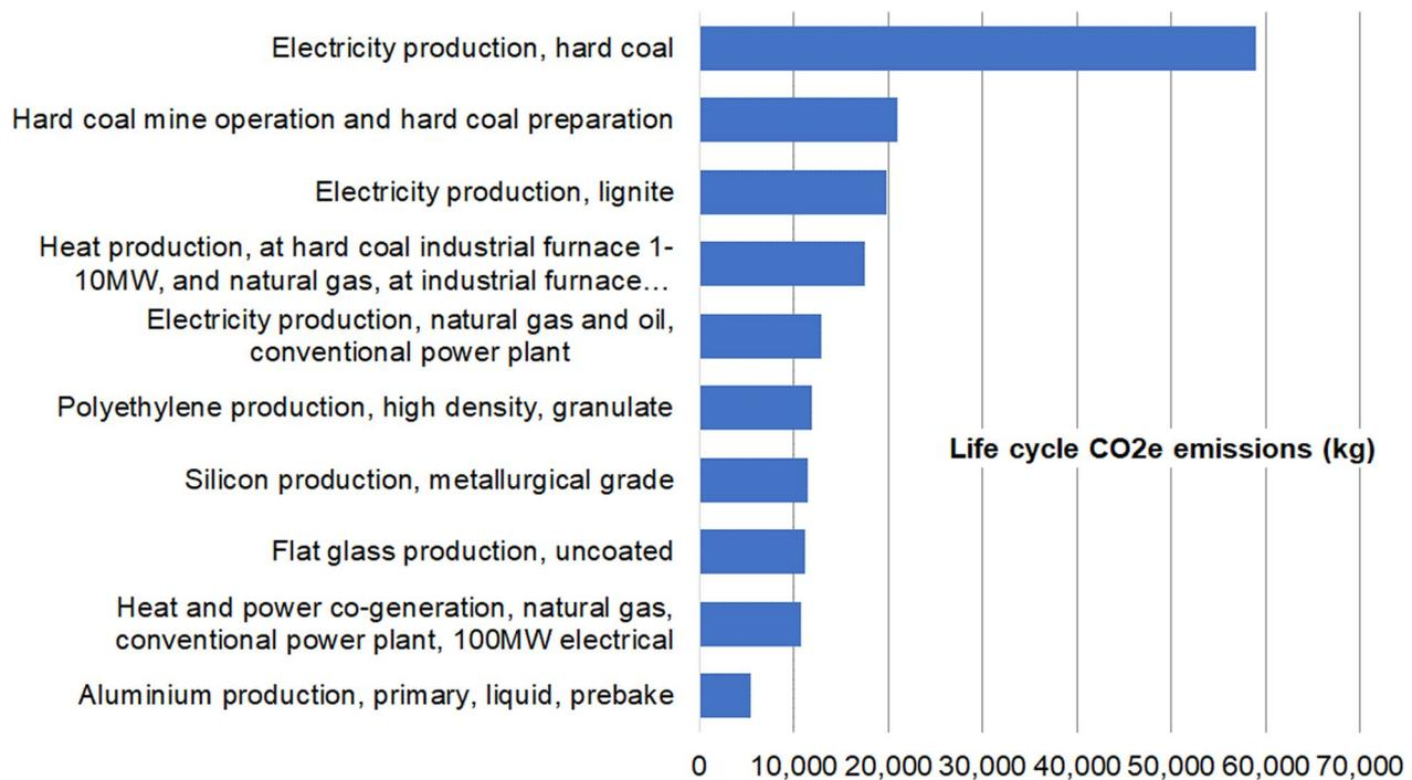
**Fig. 7** Ten most emitting processes—flat rooftop, 267 kWp multi-Si PV panel
