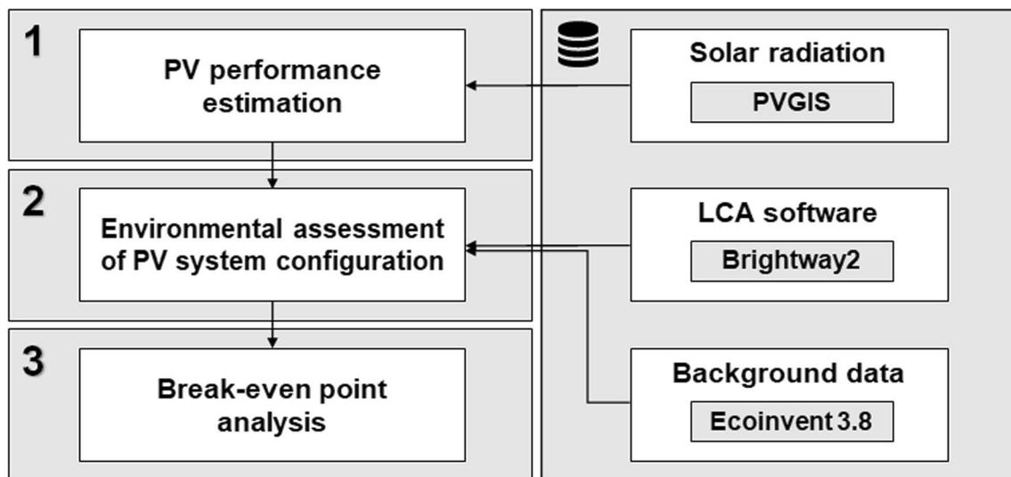
**Fig. 4** The architecture of parameterized LCA model for PV systems
